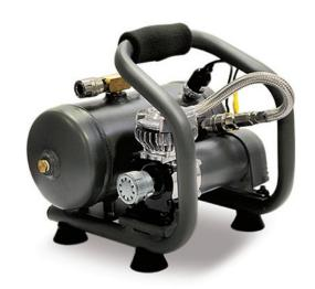
BAMBI DT500-4 is a portable air compressor that uses the DT500 series oil-free DC air compressor as the gas supply source. It can achieve continuous operation, with a maximum working pressure of 8 kilograms. Each DT500-4 is equipped with a 4-liter air storage tank, an electronic pressure switch, a one-way valve, a stainless steel braided lined PTFE hose, and a power plug that can be paired with a 12V cigarette lighter plug. It can be portable in vehicles or used in industrial applications.
